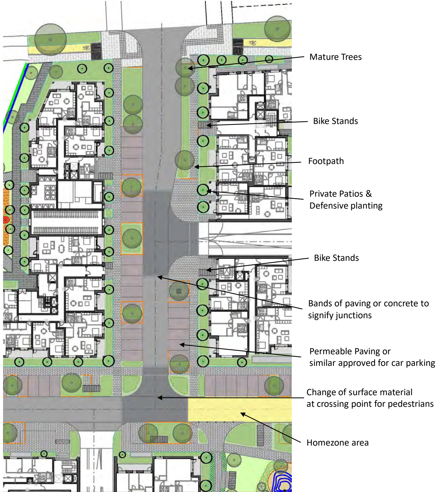
Extensive planting to provide traffic calming in the form of vertical deflection.
